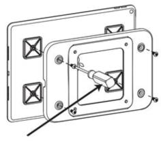
REMOVE MOUNT FROM DEVICE BY REMOVING M4 PIN TORX SCREWS USING PROVIDED T-15 SCREWDRIVER
