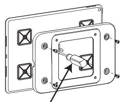
REMOVE MOUNT FROM DEVICE BY REMOVING
