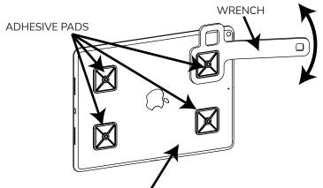
PLACE TABLET OR LAPTOP ON A FLAT PROTECTIVE SURFACE WITH THE 4 ADHESIVE PADS FACING UP. WHILE SECURELY HOLDING THE DEVICE, PLACE THE TOOL ONTO THE ADHESIVE PAD AS SHOWN AND ROTATE WITH STEADY FORCE ALLOWING THE ADHESIVE TO BREAK FREE.
